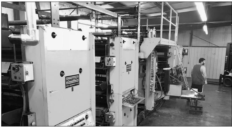
The aft-end of the press includes four more printing towers and the folder for the web press.
